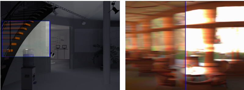
Fig. 5: Screenshots demonstrating simulation of perceptual and optical effects, possible only for HDR content. Left: simulation of night vision, resulting in a limited color vision and bluish cast of colors. Right: simulation of physically accurate motion blur (right side) compared with the motion blur computed from the traditional video material (left side).
