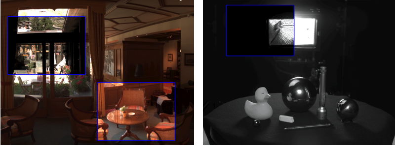
Fig. 4: Two screenshots from the advanced HDR video player, showing an extreme dynamic range captured withing HDR video sequences. Blue frames represent virtual filters that adjust exposure in the selected regions.
