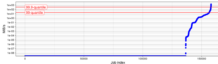
Fig. 6: Training data (subset) for read_bytes metric, and q99%- and q99.9%-quantiles (red lines).
